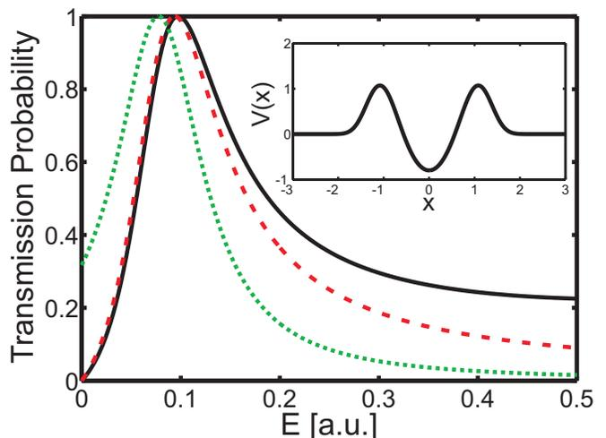
FIG. 2. (color online) The numerically exact transmission probability (solid(black) line) through a double barrier potential, see the text, using the following parameters:  $\beta = 5/2$ ,  $\gamma = 0.8$ , and  $\alpha = 0.5$ . We show only the first resonance peak. On top of the exact resonance peak we draw the BW resonance profile (dotted(green) line) (see Eq. 1) and the novel resonance profile given here (dashed(red)line) (see Eq. 2.)
