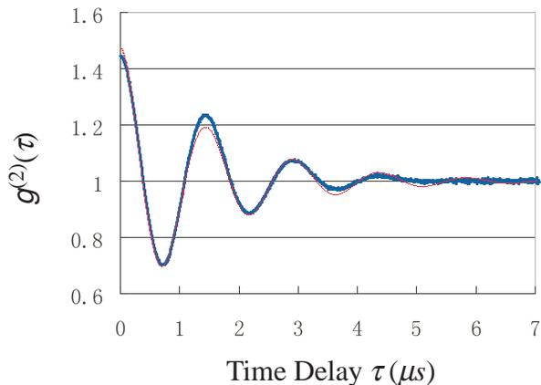
FIG. 5: Normalized intensity correlation function  $g^{(2)}(\tau)$  as function of time delay  $\tau$ . Blue line: experimental data; red line: best fitted curve to Eq.(8) with  $V = 0.47$ ,  $\gamma = 0.63\mu s^{-1}$ ,  $\Delta\nu = 0.68MHz$ .
