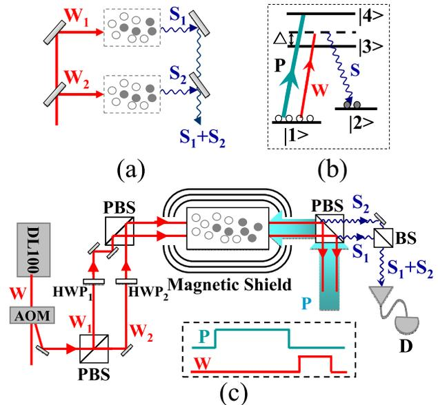
FIG. 1: (a) The conceptual diagram for the beating between two independent Stokes fields (b) Diagram for the atomic energy level and light frequencies.  $W_{1,2}$ : the Raman write fields;  $S_{1,2}$ : the generated Stokes fields. (c) Experimental layout. Inset: timing sequence.
