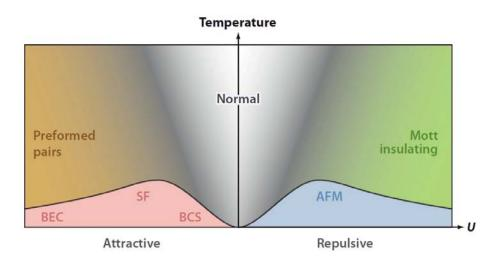
*Figure 3*: Schematic phase diagram for the attractive and repulsive Hubbard model at half filling, for a simple cubic lattice in three dimensions (see, for example Ref. (73)). Abbreviations: BEC, Bose-Einstein condensation; BCS, Bardeen-Cooper-Schrieffer; SF, superfluid; AFM, anti-ferromagnetic phase.
