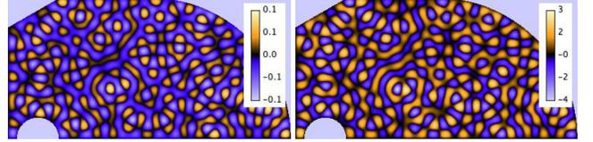
FIG. 1. Real (on the left) and imaginary (on the right) component of the 500th resonance state obtained by means of the Finite Element Method.
