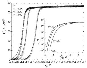
Fig. 4: The gate voltage dependence of the effective capacitance, measured at different temperatures. Inset: The gate voltage dependence of the DC conductivity at different temperatures.
