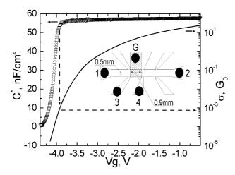
Fig. 1: The gate voltage dependence of the effective capacitance C\* in configuration 1-G. Inset: The Hall bar geometry, contacts and gate.
