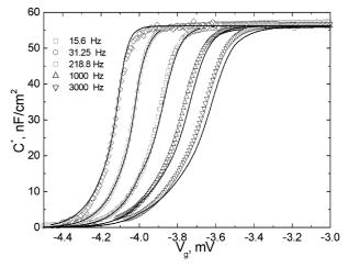
Fig. 3: The gate voltage dependence of the effective capacitance, measured at different frequencies. Solid lines show the calculated dependencies (eq. 1).
