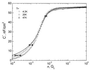
*Fig. 5: The conductivity dependence of effective capacitance C\*, measured at different temperatures.*
