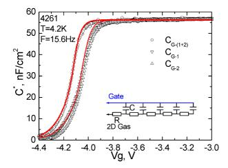
Fig. 2: The gate voltage dependencies of  $C^*$ , for all three configurations (see text for details). Solid lines (color online) show the calculated dependencies (eq. 1). Inset: The equivalent circuit for the structures investigated. In homogeneous case all the elements R and C are equal.
