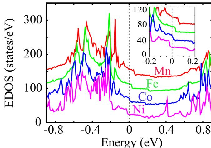
FIG. 3: (Color online) Comparison of electronic density of states (EDOS) for  $\text{La}(\text{Fe}_{0.944}\text{Mn}_{0.056})\text{AsO}$  with  $M = \text{Mn}$  (red), Fe (green), Co (blue), and Ni (pink). For each EDOS, offset values of 40 states/eV for Co, 80 states/eV for Fe, and 120 states/eV for Mn are applied. (Inset) Enlarged EDOS for the range of  $[-0.2 \text{ eV}; 0.2 \text{ eV}]$  with offset values of 20 states/eV for Co, 40 states/eV for Fe, and 60 states/eV for Mn.
