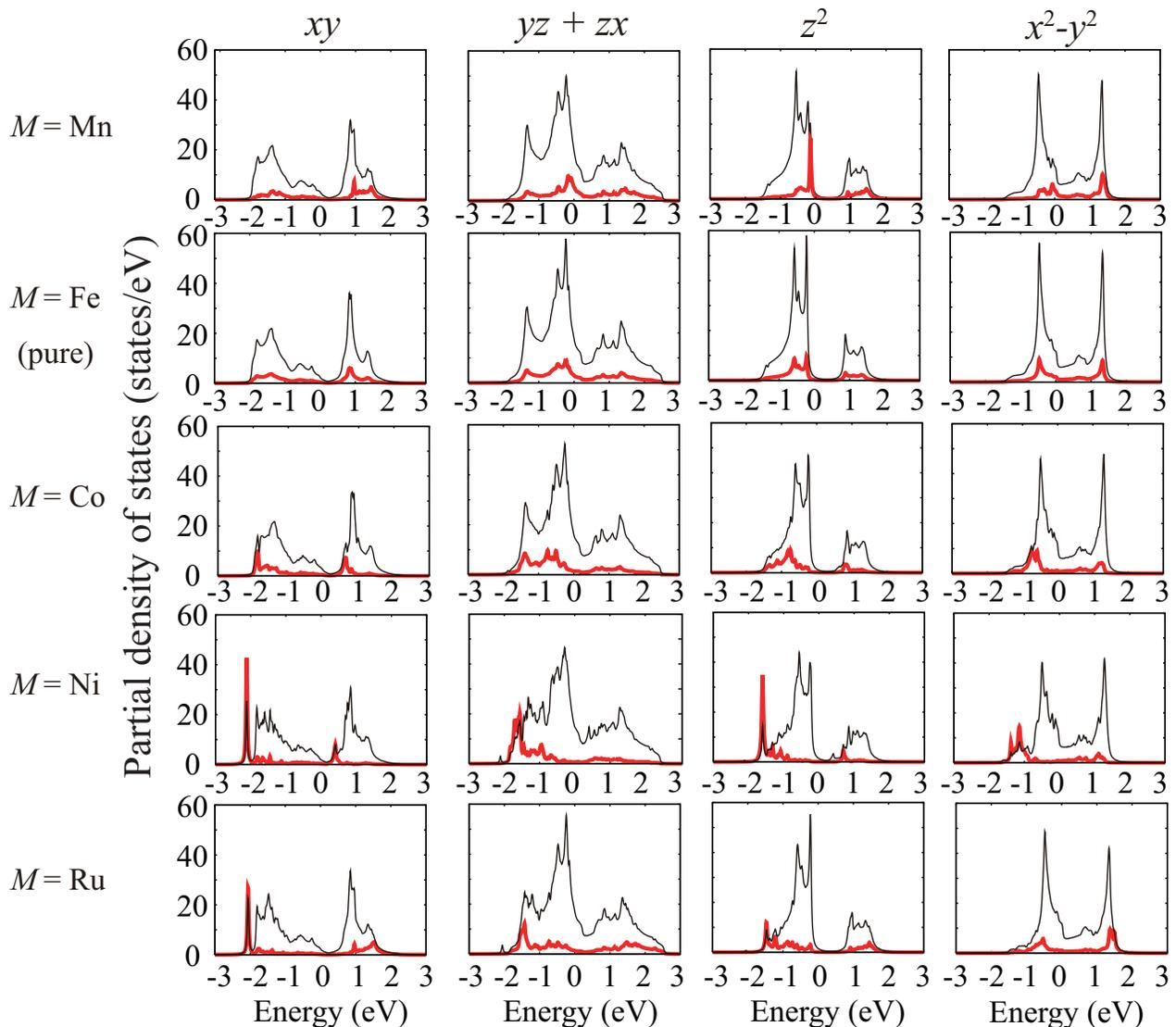
FIG. 4: (Color online) Partial density of states for  $\text{La}(\text{Fe}_{0.944}\text{M}_{0.056})\text{AsO}$  of each  $d$  orbital. From the top,  $M = \text{Mn}, \text{Fe (pure)}, \text{Co}, \text{Ni},$  and  $\text{Ru}$ . Thin-black and thick-red lines are total [Eq. (14)] and impurity [Eq. (15)] spectra, respectively. The impurity spectra are tripled. The Lorentz broadening of 0.02 eV is applied.
