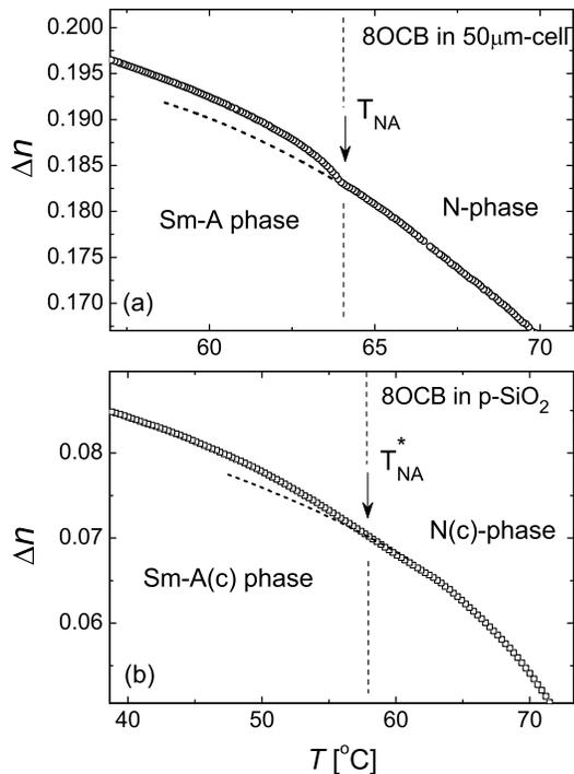
FIG. 2. Expanded plots of the temperature-dependent birefringence  $\Delta n(T)$  in the regime of the nematic-to-smectic transition: (a) bulk, (b) confined in p-SiO<sub>2</sub>.
