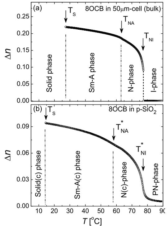
FIG. 1. Measured optical birefringence  $\Delta n$  vs. temperature  $T$  for 8OCB in the bulk state (a) and confined in 7 nm pores of p-SiO<sub>2</sub> (b).
