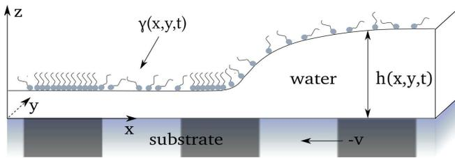
FIG. 1. Schematic drawing of a surfactant-covered meniscus on a prepatterned substrate. The height profile  $h(x, y, t)$  indicates the film thickness at location  $(x, y)$  and time  $t$ , whereas  $\gamma(x, y, t)$  describes the surfactant density at the surface above  $(x, y)$ .
