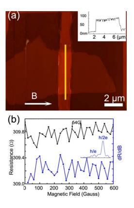
Figure 2. The MR oscillation of a broad  $Bi_2Te_3$  flake (a) The AFM image. The inset is the height profile along the marked line. It reads a cross section of  $S_2$ = 4.8µm\*73nm. The electrodes are shadowed for eye guiding. (b) MR curve (black) and
