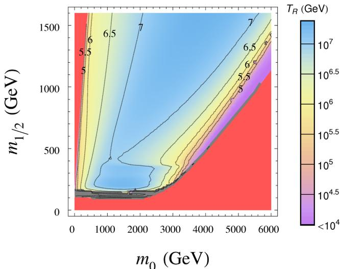
**Figure 7:** Contours of constant  $T_R$  in the  $m_0$  vs.  $m_{1/2}$  plane for  $A_0 = 0$ ,  $\tan\beta = 10$  and  $\mu > 0$ . We assume  $\Omega_a h^2 = 0.11$ , and  $\Omega_a^{TP} h^2 = 0.006$  and  $\Omega_a^{NTP} = 6 \times 10^{-6}$ .
