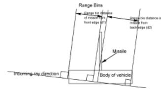
**Figure 14:** Ray diagram to show the reason for the proximity of the missile head to the front edge in SAR image.
