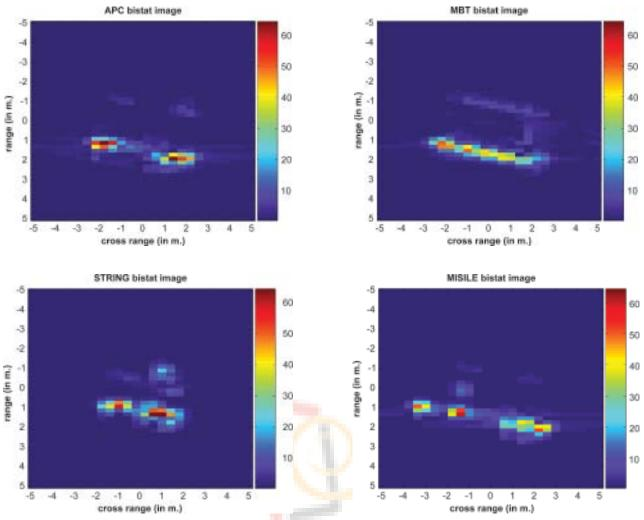
**Figure 15:** Representative bistatic SAR images of the four targets modeled (HH polarized images) (top left: APC, top right: MBT, bottom left: Missile launcher, bottom right: Stinger).
