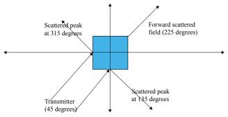
**Figure 2:** Cross section of the rectangular PEC prism, and explaining the peaks found in the bistatic RCS plot.
