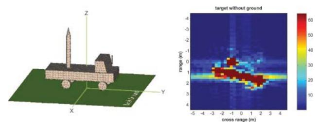
Figure 8: Optical and bistatic SAR images of the target on ground plane.
