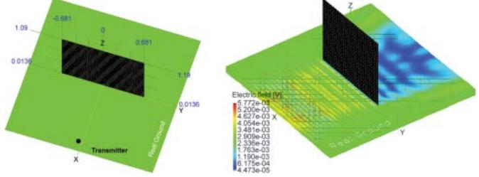
Figure 4: FEKO model of the setup and the surface current on the ground (red represents highest density of current and violet the least).
