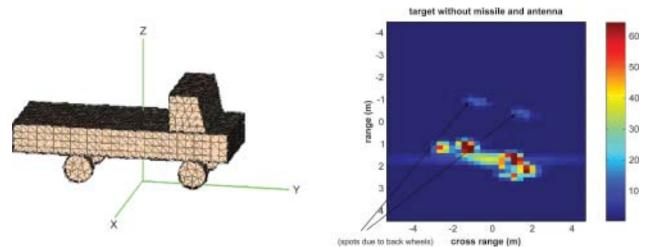
Figure 11: Optical and bistatic SAR images of the target with no missile, no antenna and no ground plane.
