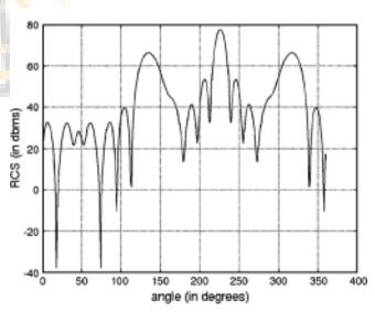
Figure 3: Bistatic RCS (in dbsm) versus azimuth angle in degrees.
