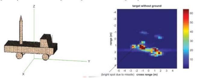
Figure 13: Optical and bistatic SAR images of the target with no ground plane.
