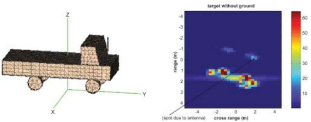
Figure 12: Optical and bistatic SAR images of the target with no missile, and no ground plane.
