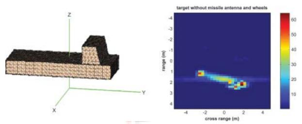
Figure 10: Optical and bistatic SAR images of the target with no wheels, no missile, no antenna and no ground plane.
