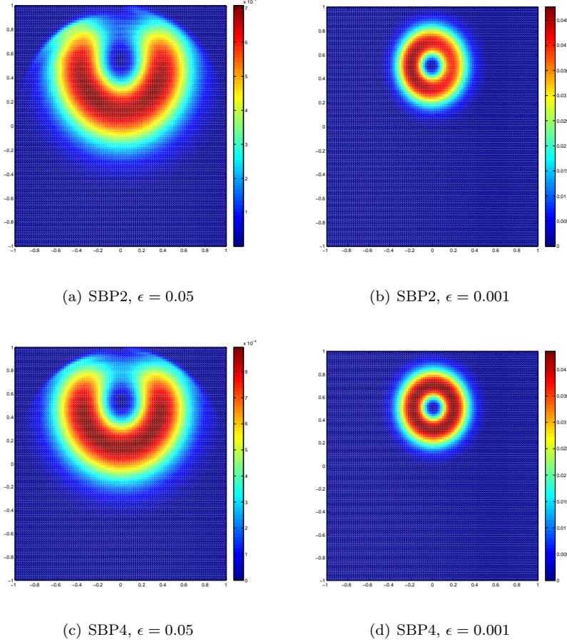
FIGURE 5.3. Numerical Experiment 3:  $|\mathbf{B}| = \sqrt{\mathbf{B}_1^2 + \mathbf{B}_2^2}$  for the SBP2 and SBP4 schemes on a  $100 \times 100$  mesh.
