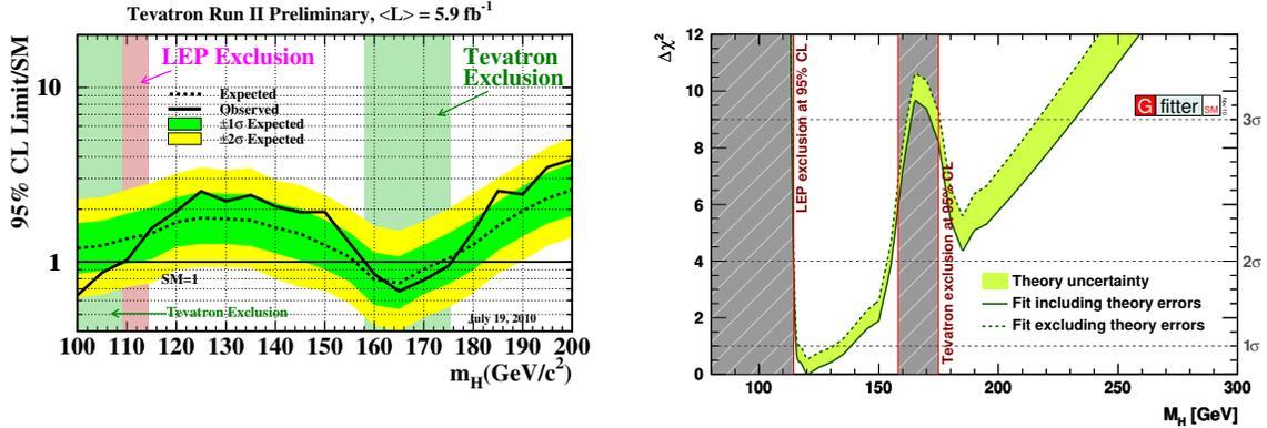
**FIGURE 2.** Searches for the Standard Model Higgs boson at the Tevatron (left) exclude the range  $158 \text{ GeV} < m_H < 175 \text{ GeV}$  [10]. Combining the Tevatron search with the LEP search [9] and the precision electroweak data[2], one obtains (right) the global  $\chi^2$  function that favours  $m_H \sim 120 \text{ GeV}$ [11].
