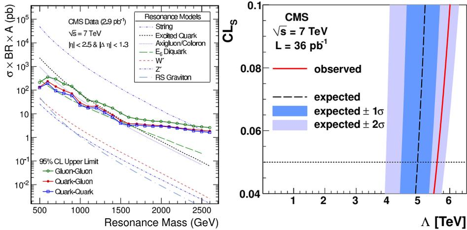
**FIGURE 10.** Left: upper limits on resonances in  $g + g$ ,  $q + g$  and  $q + q$  scattering compared with the cross sections calculated in various scenarios, note in particular the limits on excited quarks and string resonances [51] (see also [50]). Right: limit on new contact interactions scaled by  $\Lambda$ , as obtained from a study of dijet angular distributions [52] (see also [53, 54]).
