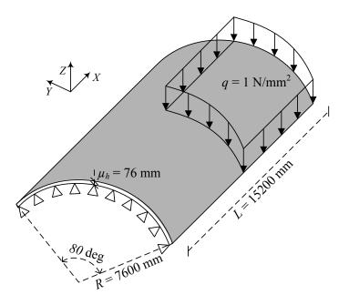
Figure 5: Illustration of the Scordelis-Lo shell roof example.
