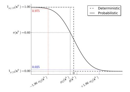
Figure 2: Comparison of the two classification strategies on a two-dimensional example from Der Kiureghian and Dakessian (1998) – Classification functions at point  $x^0$ .
