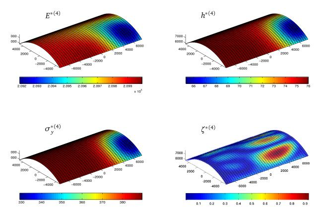
Figure 6: One of the 4 most probable failure configurations.
