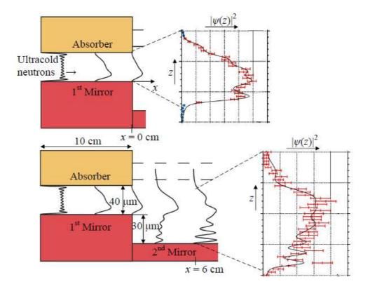
FIG. 15. (Color online) Position sensitive detection of the transmitted UCN after their "fall" over a step of 30  $\mu$ m height at the exit of the slit system, measured at two different distances from the slit exit, x = 0 cm, and x = 6 cm. This differential phase sensitive measurement of neutron transmission in principle is much more sensitive to fifth forces than is the integral transmission curve, Fig. 14. Adapted from Jenke *et al.* (2009).
