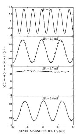
FIG. 6. The "dressed neutron" effect can be used in EDM searches to suppress unwanted magnetic effects. Spin precession about a static magnetic field  $B_0$  can be suppressed when the neutrons are irradiated with a strong radio frequency field  $B_1$  of arbitrary frequency. With RF amplitude increasing from the top to the bottom of the figure, spin-precession of the dressed neutrons slows down, then comes to a full stop, and reverses its sign. From Muskat *et al.* (1987).
