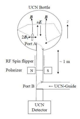
FIG. 5. Sketch of the Ramsey apparatus used at ILL to search for a neutron electric dipole moment (nEDM). The block arrow shows the neutron polarization right after filling of the UCN trap (Port A and B open). The dashed line represents a UCN trajectory in the UCN bottle. The sources of the **E** and **B** fields are not shown.
