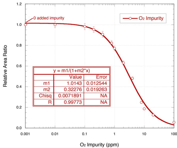
**Figure 21.** Ratio of contaminated argon pulse area to pure argon pulse area for increasing ppm O<sub>2</sub> impurity concentrations in liquid argon. The data were fitted with a Birk's law type function, where  $m1 = 1.01 \pm 0.01$  and  $m2 = 0.32 \pm 0.02$ .
