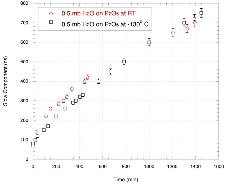
**Figure 14.** Efficiency of phosphorous pentoxide at room temperature and  $-130^{\circ}\text{C}$  at removing 0.5 mbar  $\text{H}_2\text{O}$  partial pressure impurity in 1 bar  $\text{N}_6$  argon gas.
