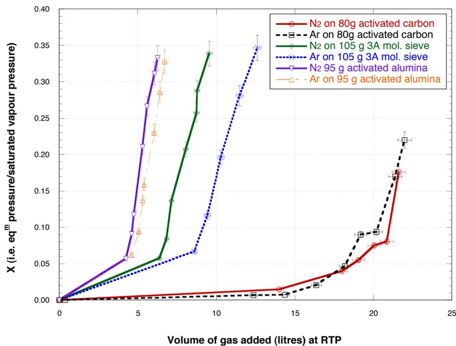
**Figure 9.** Adsorption of nitrogen and argon gas on a range of adsorbents and molecular sieves as a function of added gas. Lines are present to illustrate trends and do not indicate a fit to the data.
