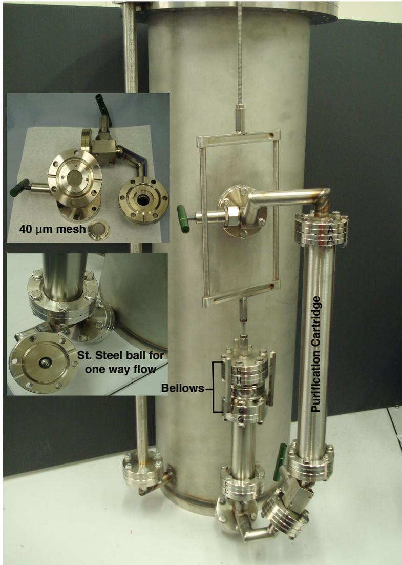
**Figure 17.** The target vessel and re-circulation system.
