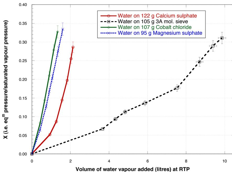
**Figure 11.** Adsorption of water vapour on a range of adsorbents and molecular sieves as a function of added water. Lines are present to illustrate trends and do not indicate a fit to the data.
