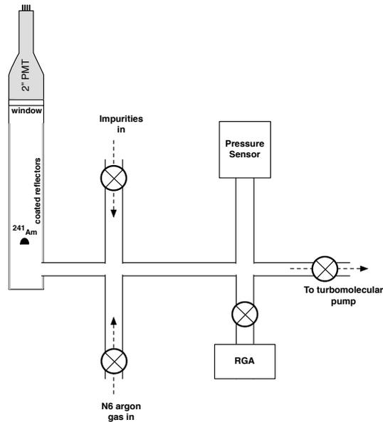
**Figure 2.** A schematic illustration of the experimental apparatus used to measure the effect of electronegative impurities on gaseous argon scintillation light.
