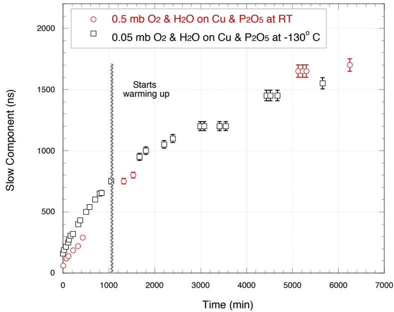
**Figure 15.** Efficiency of copper and phosphorous pentoxide mixture at both room temperature and  $-130^{\circ}\text{C}$  at removing 0.5 mbar and 0.05 mbar respectively  $\text{O}_2/\text{H}_2\text{O}$  partial pressure impurity in 1 bar  $\text{N}_6$  argon gas. The vertical black line indicates the point at which the purification mixture started to warm up.
