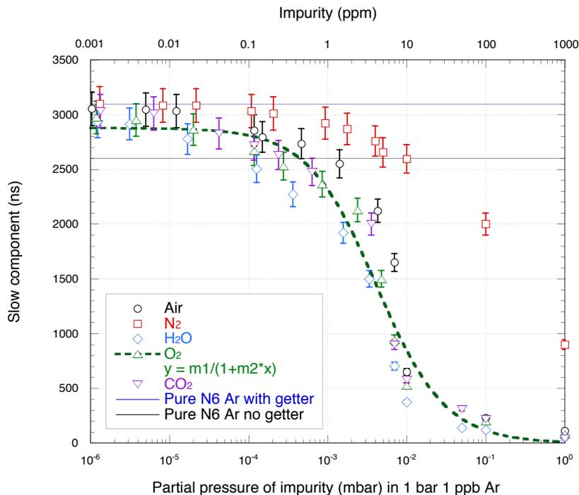
**Figure 6.** Argon gas purity: Slow component (triplet) decay time variation with contaminant partial pressure. The O<sub>2</sub> data were fitted with a Birk's law type function, where  $m1 = 2878 \text{ ns} \pm 80 \text{ ns}$  and  $m2 = 0.24 \pm 0.03$ .
