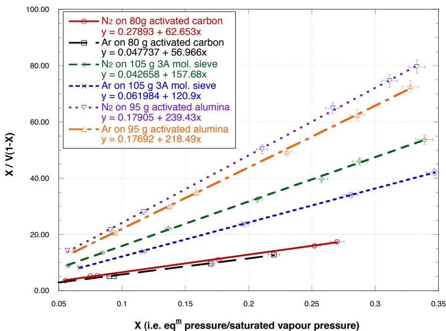
**Figure 8.** Adsorption of nitrogen and argon gas on a range of adsorbents and molecular sieves.
