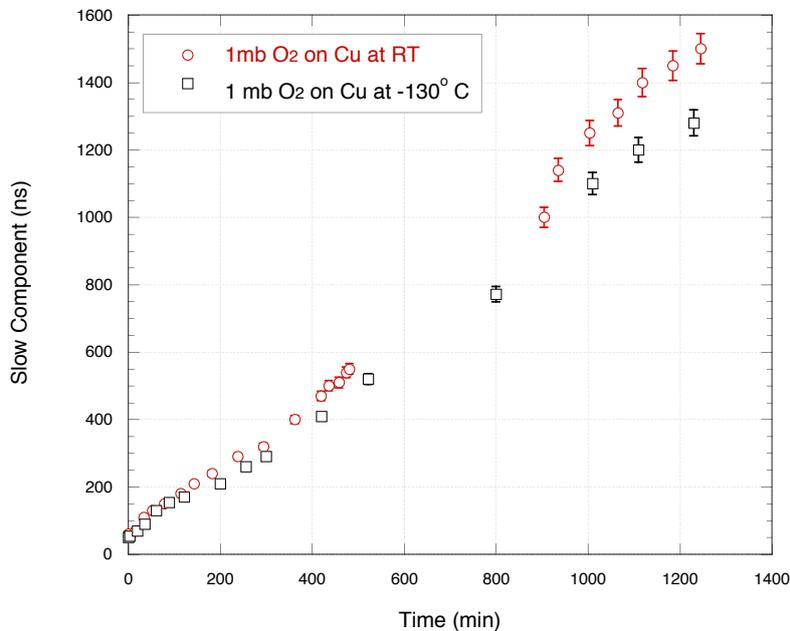
**Figure 13.** Efficiency of copper at room temperature and -130 °C at removing 1 mbar O<sub>2</sub> partial pressure impurity in 1 bar N6 argon gas.
