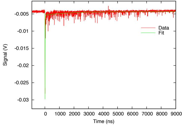
**Figure 1.** A typical argon gas scintillation pulse.
