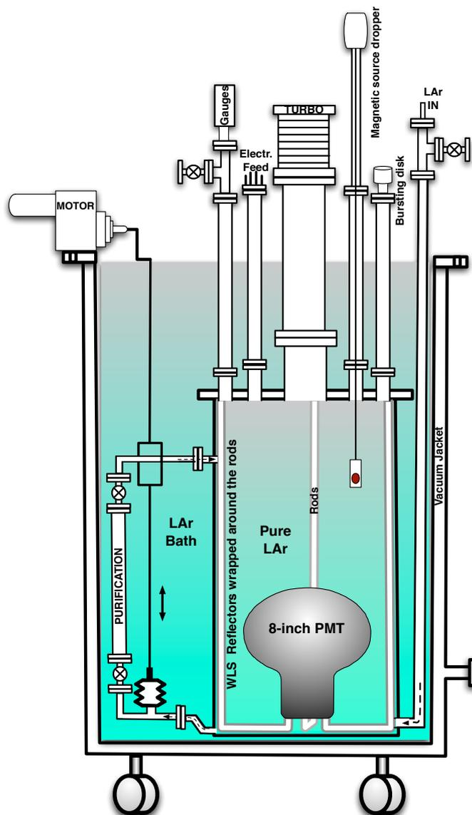
**Figure 16.** A schematic of the Liverpool LAr setup.
