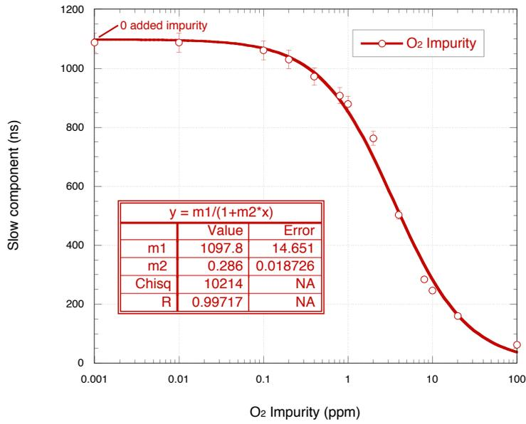
**Figure 20.** Slow component (triplet) decay time variation with increasing ppm O<sub>2</sub> impurity concentrations in liquid argon. The data were fitted with a Birk's law type function, where  $m1 = 1098 \text{ ns} \pm 15 \text{ ns}$  and  $m2 = 0.29 \pm 0.02$ . The slow component observed at 1 ppm impurity corresponds well to that observed for liquified N6 argon gas (Figure 18).
