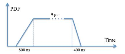
The low-band filter of 8 MHz will distort the leading and trailing edges with a time constant of 1/8,000,000 = 125 ns as shown schematically here:
