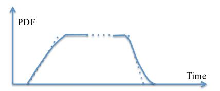
The precise shape will depend on the filtering algorithm used. A deformation of the PDF edges by 125 ns will certainly have an impact on the total anomaly of 60 ns.
