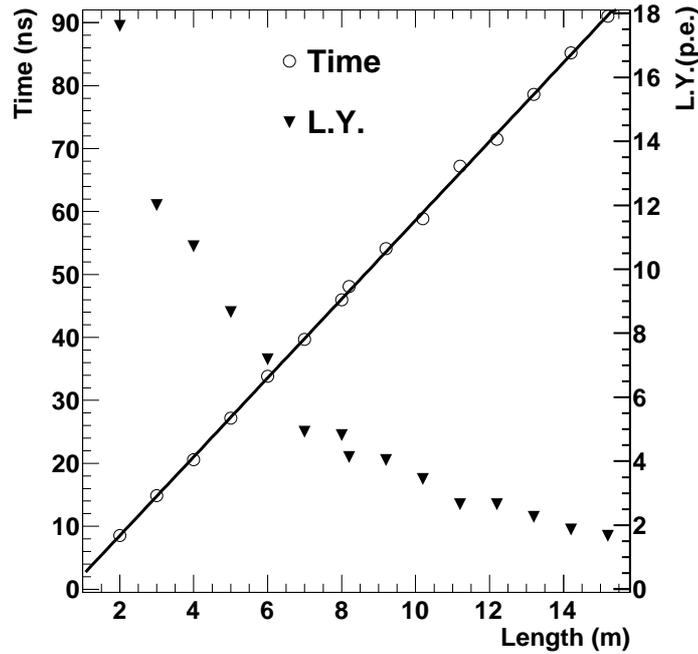
FIG. 7: Time difference between the trigger signal and the signal from the MRS APD along a 16 m long Y11 fiber of 1 mm diameter. The timing error of  $\pm 0.3$  ns is within the radius of the open circles. The light yield in photoelectrons per a minimum ionizing particle is also plotted.
