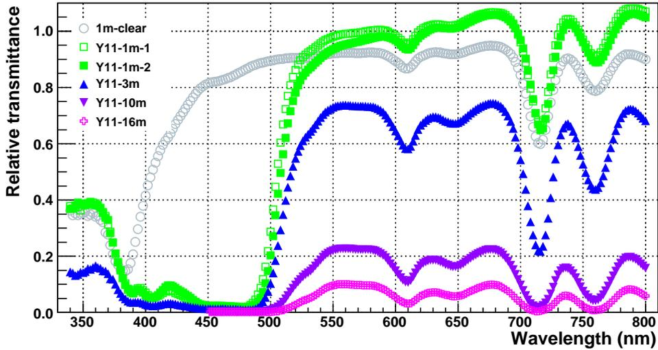
FIG. 3: Relative spectral transmittance of 1 m (two samples), 3 m, 10 m and 15 m long Y11 Kuraray fibers. Transmittance is equal to 1.0 at all wavelengths for a 10 cm long reference clear fiber.
