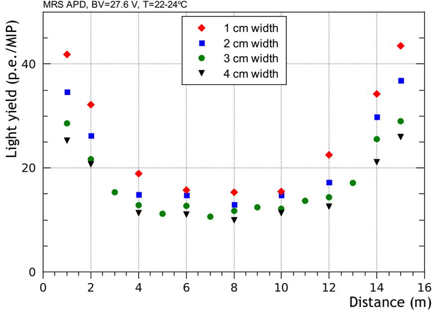
FIG. 9: Total light yield from both fiber ends vs the position along the Y11 fiber for 0.7 cm thick bars of different widths. Measurement errors are estimated to be about 7%.
