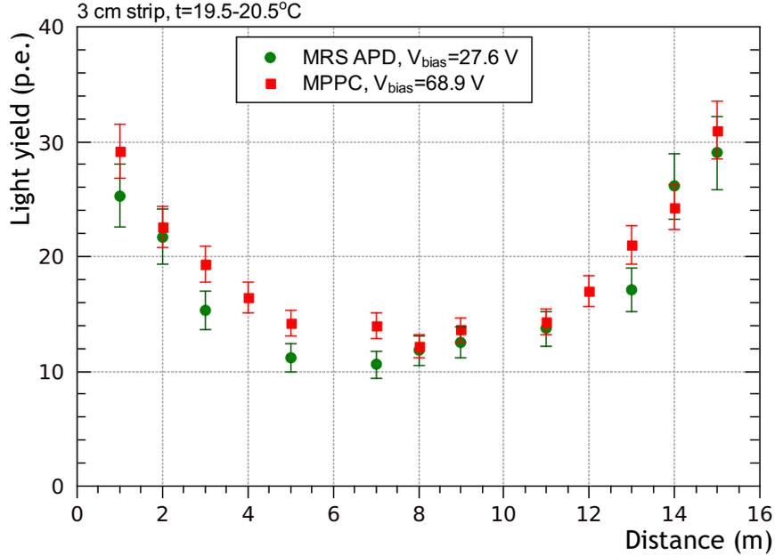
FIG. 10: Light yield (sum of both ends) along the Y11 fiber for the 3 cm wide bar read out with MRS APDs and MPPCs.
