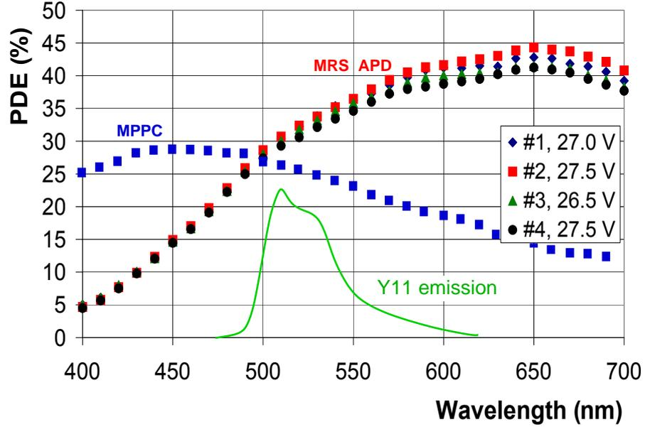
FIG. 2: Photon detection efficiency as a function of wavelength for 4 samples of MRS APDs and an MPPC at 25°C. The bias voltage for each MRS APD was set to an overvoltage of  $\Delta V=2$  V for all tested samples. MPPC was measured at  $\Delta V=1.2$  V. Also shown is the Y11(150) Kuraray fiber emission spectrum (in arbitrary units) for a fiber length of 150 cm (Kuraray specification).
