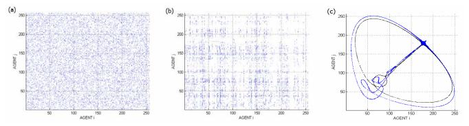
Figure 2. Ten thousand pairs of one byte integers produced the chaotic number generator (a) random integers produced with P=45. (b) random integers of poor statistical quality with P=3. (c) two sets of chaotic integers produced with two sets of control parameters  $\lambda_A = \lambda_B = 1.05032$  (black line) and  $\lambda_A = 1.05032 \lambda_B = 1.08492$  (blue line).
