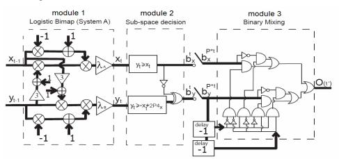
Figure 1. Functional structure of the chaotic number generator used in the experiment.
