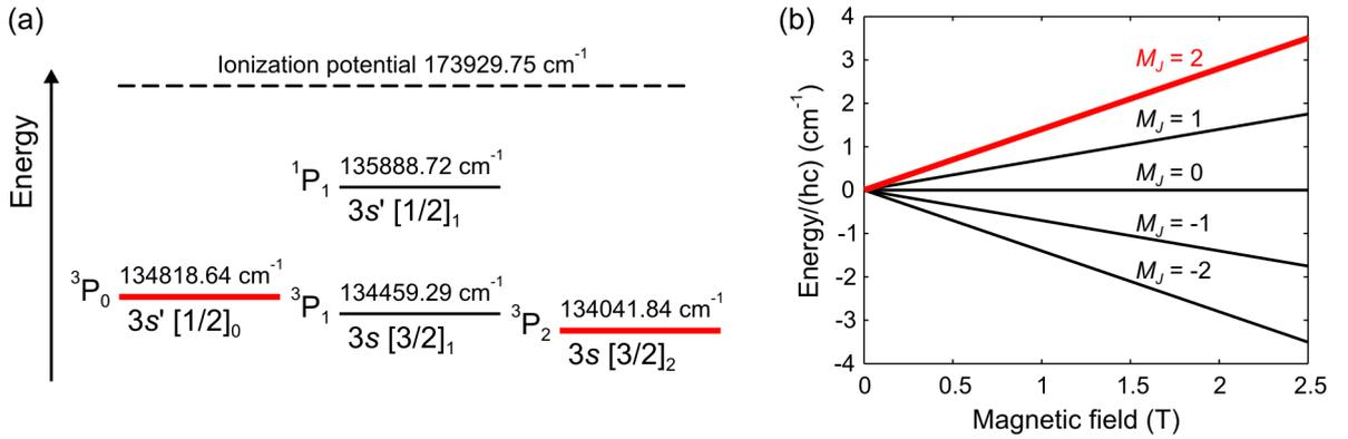
FIG. 1. (a) Schematic energy level diagram of the states of Ne relevant to the experiment, with wave numbers given relative to the  $(2p)^6\ ^1S_0$  ground state [50]. The metastable states  $^3P_2$  and  $^3P_0$  are indicated by thick red lines. (b) Zeeman effect in the  $^3P_2$  state. The low-field-seeking state  $M_J = 2$  with the largest magnetic moment is depicted in red.
