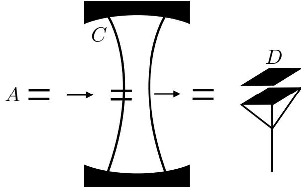
FIG. 2. Illustration of a possible experimental setup realizing a forced harmonic oscillator weakly coupled to a thermal reservoir. A sequence of two level-atoms,  $A$ , pass through a cavity  $C$ , after which their final state is measured by detector  $D$ .
