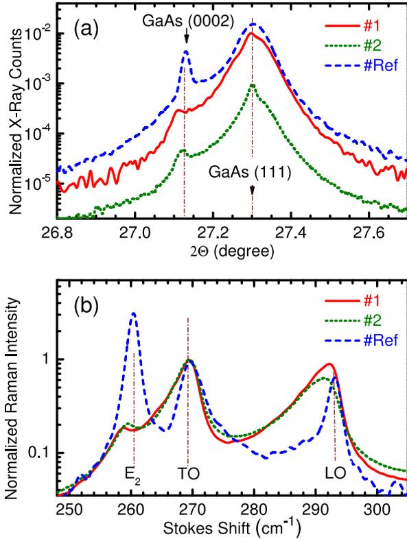
FIG. 2. (Color online) (a)  $\omega$ - $2\theta$  scans and (b) Raman spectra of the as-grown samples #1 and #2 as well as of the reference sample. In (b),  $E_2$  and TO (LO) indicate the corresponding phonon lines of GaAs where the  $E_2$  phonon mode exists only in the WZ phase.
