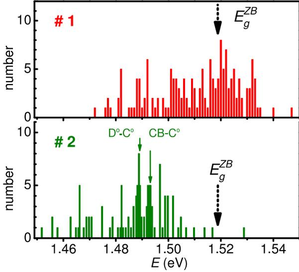
FIG. 4. (Color online) Histogram of peaks found in the  $\mu$ PL spectra of 30 NWs from samples #1 and #2 dispersed on Si(111) as a function of the respective spectral position.  $E_g^{ZB}$  marks the band gap energy of zincblende GaAs.  $D^{\circ}-C^{\circ}$  and  $CB-C^{\circ}$  mark the energy position of the donor-acceptor pair and conduction-band-acceptor transition with carbon acting as acceptor. The corresponding  $\mu$ PL spectra have been measured at 10 K.
