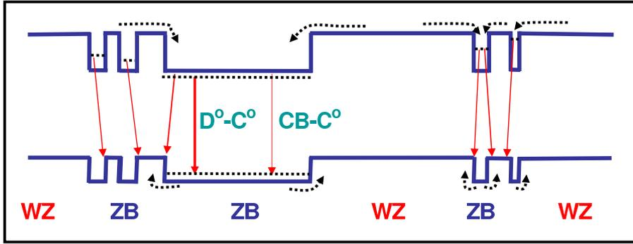
FIG. 9. (Color online) Qualitative model of the band gap alignment for samples #1 and #2. ZB and WZ mark zincblende and wurtzite GaAs segments, respectively. CB-C<sup>o</sup> and D<sup>o</sup>-C<sup>o</sup> mark conduction-band-acceptor (carbon) and donor-acceptor (carbon) transitions, respectively.
