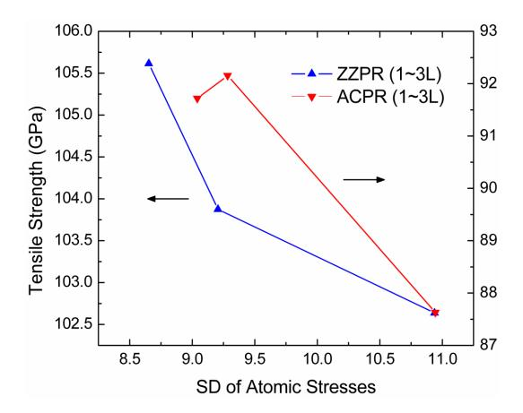
**Figure 5.** The relationship between SD of atomic stress and tensile strength for ZZ-nL and AC-nL systems (n=1~3).
