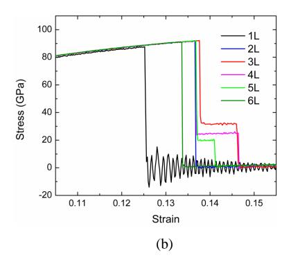
**Figure 3.** The enlarged stress-strain curves around tensile failure for various FLGs and MLG under (a) zigzag-directional elongations and (b) armchair-directional elongations.
