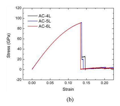
**Figure 2.** The stress-strain curves of (a) 1~3 layer (denoted as AC-1L, AC-2L, and AC-3L respectively) and (b) 4~6 layer (denoted as AC-4L, AC-5L, and AC-6L, respectively) graphene sheets under armchair-directional elongations.
