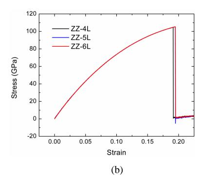
**Figure 1.** The stress-strain curves of (a) 1~3 layer (denoted as ZZ-1L, ZZ-2L, and ZZ-3L, respectively) and (b) 4~6 layer (denoted as ZZ-4L, ZZ-5L, and ZZ-6L, respectively) graphene sheets under zigzag-directional elongations.
