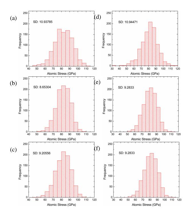
**Figure 4.** The atomic stress distributions of (a) ZZ-1L, (b) ZZ-2L, (c) ZZ-3L, (d) AC-1L, (e) AC-2L, and (f) AC-3L systems at the stages corresponding to tensile stress of 80 GPa. For 2L and 3L systems, the frequency is reduced by dividing the original frequency by one and two, respectively, for the comparison. SD denotes standard deviation.
