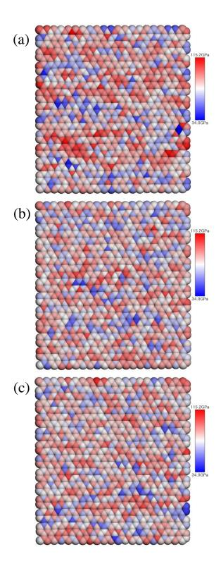
**Figure 6.** The spatial atomic stress distributions of (a) AC-1L, (b) an upper layer of AC-2L, and (c) a lower layer of AC-2L.
