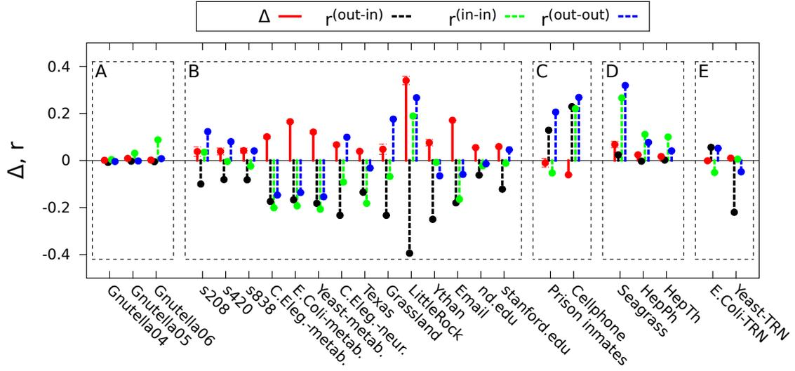
FIG. 7. The observed and predicted deviation between  $N_D$  and  $N_D^{\text{rand}}$ . Red line:  $\Delta = (N_D - N_D^{\text{rand}})/N$ , the prediction error based on the degree sequence. Dashed lines: correlations relevant to controllability. For each network  $\Delta$  is calculated by averaging over 50 independent configurations.
