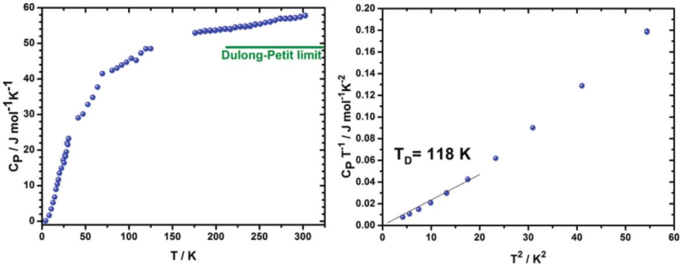
FIG. 3: (left) Specific heat capacity of spark plasma sintered PbTe nanoparticles. (Right) Plot of  $C_P/T$  vs  $T^2$  to derive the Debye temperature of a pellet of spark plasma sintered PbTe nanoparticles.
