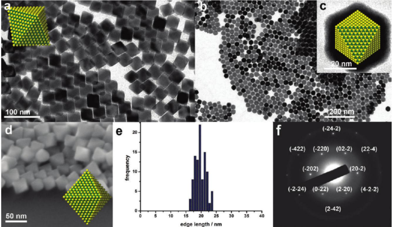
FIG. 1: (a-c) TEM images of octahedral PbTe nanoparticles in (a)  $<110>$ - and (b and c)  $<111>$ -projection. (d) SEM image of PbTe nanoparticles. (e) Histogram of the PbTe nanoparticles' edge lengths. (f) SAED of the single PbTe nanoparticle in panel c. Indexing is according to the rock salt structure.
