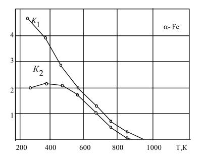
**Figure**. Temperature dependence of the magnetic anisotropy constants of the  $\alpha - Fe$
