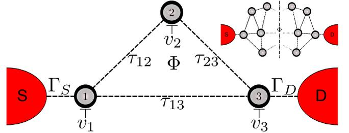
FIG. 1. (Color online) Three quantum dots in a ring arrangement, with dots 1 and 3 connected to the source  $S$  and drain  $D$  via tunneling rates  $\Gamma_S$  and  $\Gamma_D$ , respectively. Dot  $i$  is subject to a local potential  $v_i$  (taken here to be  $v_i = 0$ ). The lowest single-particle orbitals of dots  $i$  and  $j$  are connected via tunnel couplings  $\tau_{ij}$ . The ring is threaded by a flux  $\Phi$ . Inset: A reflection-symmetric Aharonov-Bohm network.
