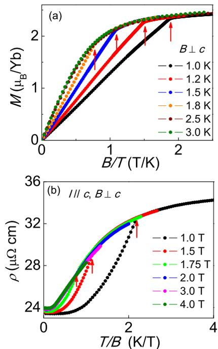
FIG. 6: (Color online) (a) Field dependencies of the magnetization  $M$  were measured at different temperatures, and then plotted as functions of  $B/T$ . (b) The temperature dependencies of the electrical resistivity  $\rho$  were measured in different magnetic fields from 1.0 T to 4.0 T, and then plotted as functions of  $T/B$ . Red arrows indicate the onset of antiferromagnetic order, showing that the resistivity data collapse onto a single curve in the paramagnetic phase.
