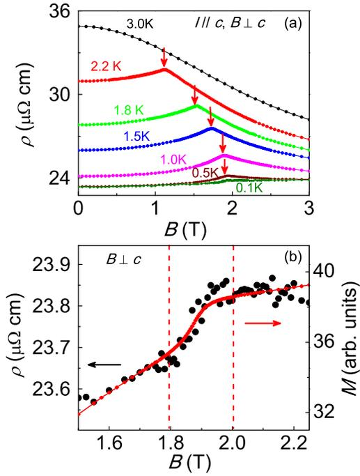
FIG. 3: (Color online) (a) Field dependencies of the electrical resistivity  $\rho$  measured at different temperatures from 0.1 K to 3.0 K, as indicated. Red arrows indicate the antiferromagnetic transitions. (b) Magnetoconductivity  $\rho$  ( $\bullet$ , left axis) measured at 0.1 K plotted together with the magnetization (red solid line, right axis) measured at 0.2 K. Vertical dashed lines delineate the step like kink around the critical field  $\sim 1.85$  T.
