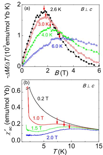
FIG. 8: (Color online) (a)  $-\Delta M/\Delta T$  vs  $B$  calculated as described in the text, for different fixed temperatures. (b) The temperature dependencies of the real part of the ac magnetic susceptibility  $\chi'_{ac}$ , measured at different fields. The red arrows in (a) and (b) mark the positions of maxima.
