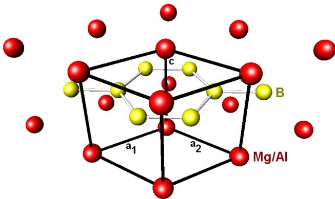
Figure 1. (Color online) Unit cell of  $Mg_xAl_{1-x}B_2$ . The red and yellow spheres correspond to the (Mg,Al) and B sites. In its space group  $P6/mmm$  magnesium/aluminum and boron reside on special positions at  $0,0,0$  and  $\frac{1}{3}, \frac{2}{3}, \frac{1}{2}$ , respectively. The B rings and the intercalated Mg sheets have a hexagonal atomic arrangement and are stacked alternately along the  $c$  axis.
