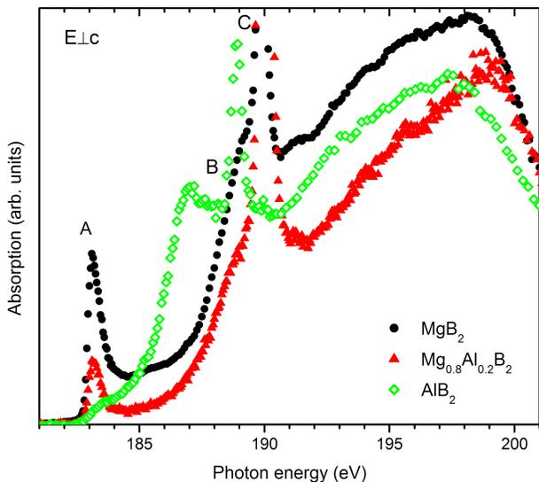
Figure 4. (Color online) Orbital-specific electronic structure of single-crystalline  $\text{MgB}_2$ ,  $\text{Mg}_{0.8}\text{Al}_{0.2}\text{B}_2$ , and  $\text{AlB}_2$ : B  $1s$  NEXAFS with  $\mathbf{E}\perp\mathbf{c}$ , probing unoccupied  $\sigma$ -bonded B  $2p_{xy}$  and  $\pi$ -bonded B  $2p_z$  states.
