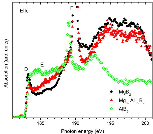
Figure 5. (Color online) Orbital-specific electronic structure of single-crystalline  $\text{MgB}_2$ ,  $\text{Mg}_{0.8}\text{Al}_{0.2}\text{B}_2$ , and  $\text{AlB}_2$ : B  $1s$  NEXAFS with  $\mathbf{E}\parallel\mathbf{c}$ , probing unoccupied  $\pi$ -bonded B  $2p_z$  states.
