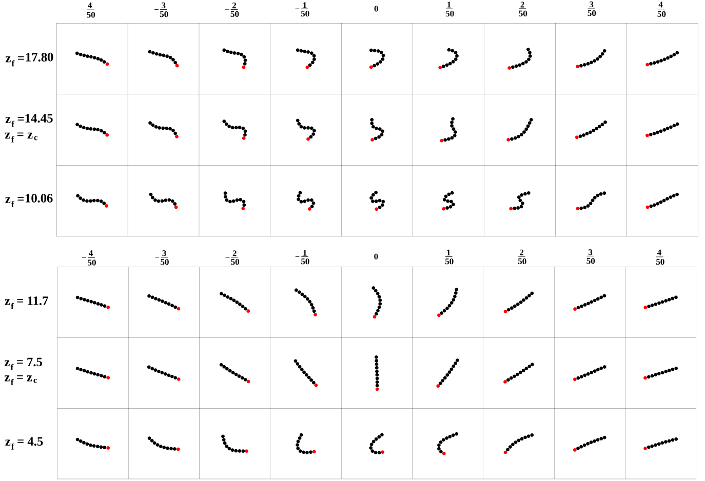
Fig. 6. Evolution of a fiber shape (drawn to scale) for N = 10 . Up: A = 0.2 . Down: A = 1 . Snapshots from simulations taken at the indicated times \bar{t}/\tau (with \bar{t} = t - t_f(2) and \tau = t_f(3) - t_f(2) , where t_f(n) is the instant of the n -th flip). The indicated values of z_f are attained at \bar{t} = 0 (second flip).
