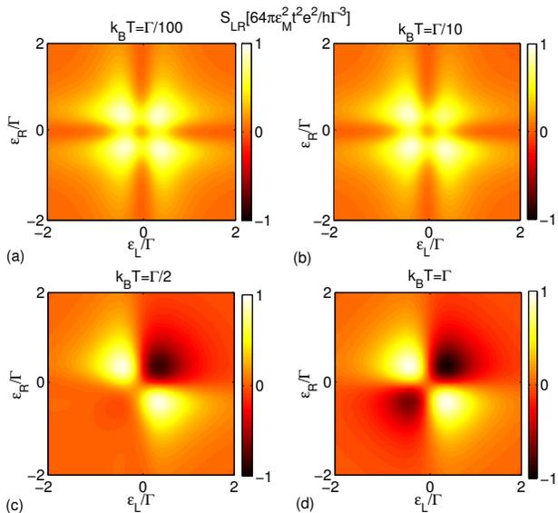
FIG. 5. (color online) Finite temperature current cross correlations  $S_{LR}$  for strong dot-lead coupling with  $eV = \Gamma/2$ ,  $t = \Gamma/20$ ,  $\epsilon_M = \Gamma/10$ , and  $\Delta = 0$ . (a)  $k_B T = 0$ , (b)  $k_B T = \Gamma/10$ , (c)  $k_B T = \Gamma/2$ , and (d)  $k_B T = \Gamma$ .
