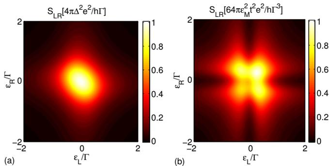
FIG. 4. (color online) Current cross-correlator  $S_{LR}$  for  $eV = \Gamma/2$ . The dots are coupled (a) via the SC proximity effect with  $\Delta = \Gamma/10$  and (b) via SC proximity effect and with coupling to a pair of MBS with  $t = \Gamma/20$ ,  $\Delta = \Gamma/20$ , and  $\epsilon_M = \Gamma/10$ .
