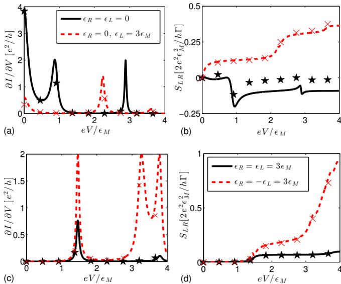
FIG. 2. (color online) Current cross-correlator  $S_{LR}$  in the weak dot-lead coupling regime with  $\Gamma = \epsilon_M/4$ ,  $t = 0.8\epsilon_M$ , and  $\Delta = 0$ . The lines for panel (b) are defined in (a), those for panel (c) in (d). The markers denote the results for the spinless SC model with  $\epsilon_M = 0.01$  meV and  $\Gamma = 0.002$  meV.
