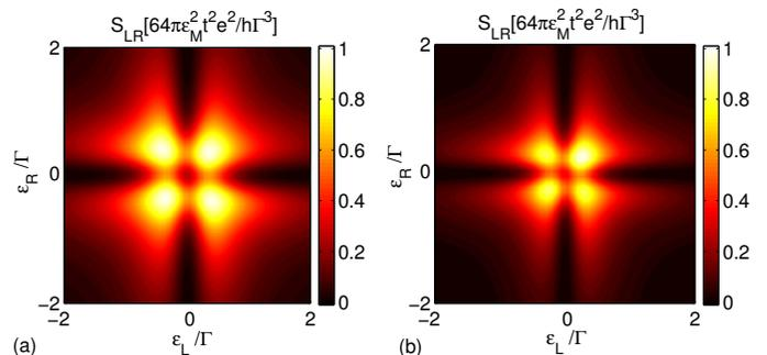
FIG. 3. (color online) Current cross-correlator  $S_{LR}$  for strong dot-lead coupling. (a) Effective model with  $eV = \Gamma/2$ ,  $t = \Gamma/20$ ,  $\epsilon_M = \Gamma/10$ , and  $\Delta = 0$ . (b) Spinless SC with  $\epsilon_M = 0.01$  meV and  $\Gamma = 0.06$  meV. For both (a) and (b), the pattern changes little for larger  $eV$ .
