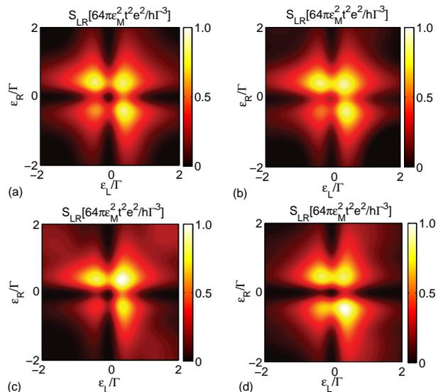
FIG. 10. (color online) Current cross correlations  $S_{LR}$  of the single-band semiconductor model with  $\mu_0 = 0$  for different disorder strengths. Ensemble averaged cross noise for disorder strengths (a)  $U = \Delta/4$  and (b)  $U = \Delta/2$ . Crossed noise for a characteristic disorder realization with (c)  $U = \Delta/4$  and (d)  $U = \Delta/2$ .
