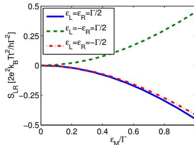
FIG. 6. (color online) Current cross-correlations  $S_{LR}$  for strong dot-lead coupling with  $eV = \Gamma/2$ ,  $t = \Gamma/20$ ,  $\epsilon_M = \Gamma/10$ ,  $\Delta = 0$ , and  $T = \Gamma$  as function of the Majorana energy splitting  $\epsilon_M$ .
