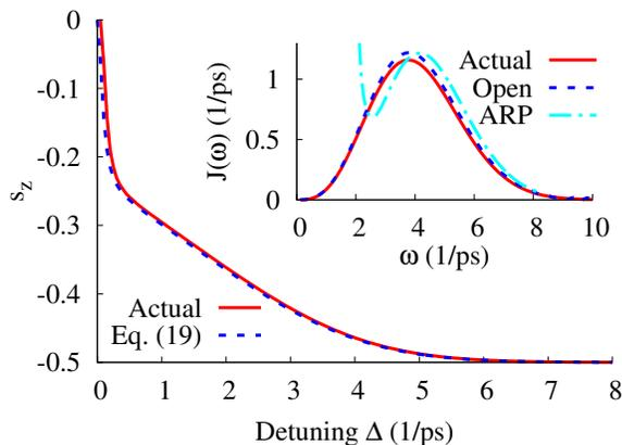
FIG. 8. (color online). Main figure: Steady-state value of  $s_z$  with driving at  $\Omega = 0.1 \text{ ps}^{-1}$ , with a spontaneous decay rate of  $\kappa = 2 \text{ ns}^{-1}$ , as a function of the detuning, at  $T = 20 \text{ K}$ . Inset: comparison of actual phonon density of states  $J(\omega)$  with the values reconstructed by inverting Eq. (19) and from the modified ARP approach, inverting Eq. (15) (parameters for modified ARP as in Fig. 7).
