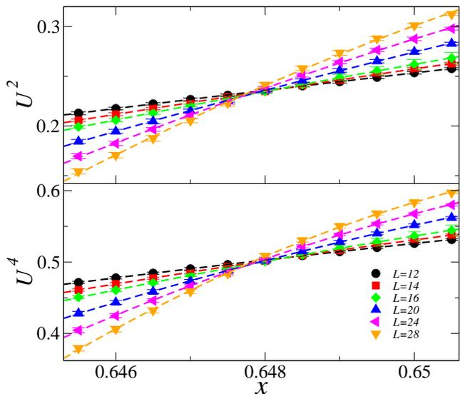
FIG. 1: (color online) Curve crossings for the second (upper graph) and fourth (lower graph) order cumulants for various lattice sizes as function of the control parameter  $x$ . The crossing region is the same in both cases. Dashed lines are third order polynomial fittings.
