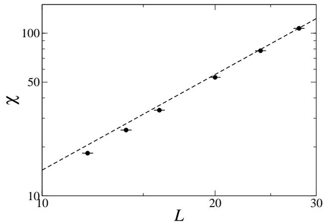
FIG. 4: Log-log plot of the susceptibility at the critical point as function of the linear dimension  $L$ . The dashed lines show the expected power law behavior in the  $L \rightarrow \infty$  limit with  $\gamma/\nu = 1.952$ .
