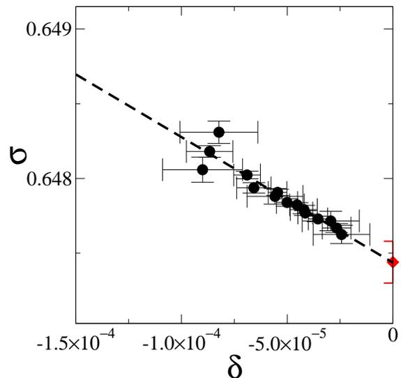
FIG. 2: (color online) Evaluation of the critical point using the quantities  $\sigma = (x_{ij}^4 + x_{ij}^2)/2$  and  $\delta = x_{ij}^4 - x_{ij}^2$ , where  $x_{ij}^q$  is the crossing point between cumulants  $U^q$  for linear sizes  $L_i$  and  $L_j$ . The dashed line is the linear fit and the red diamond shows the critical point.
