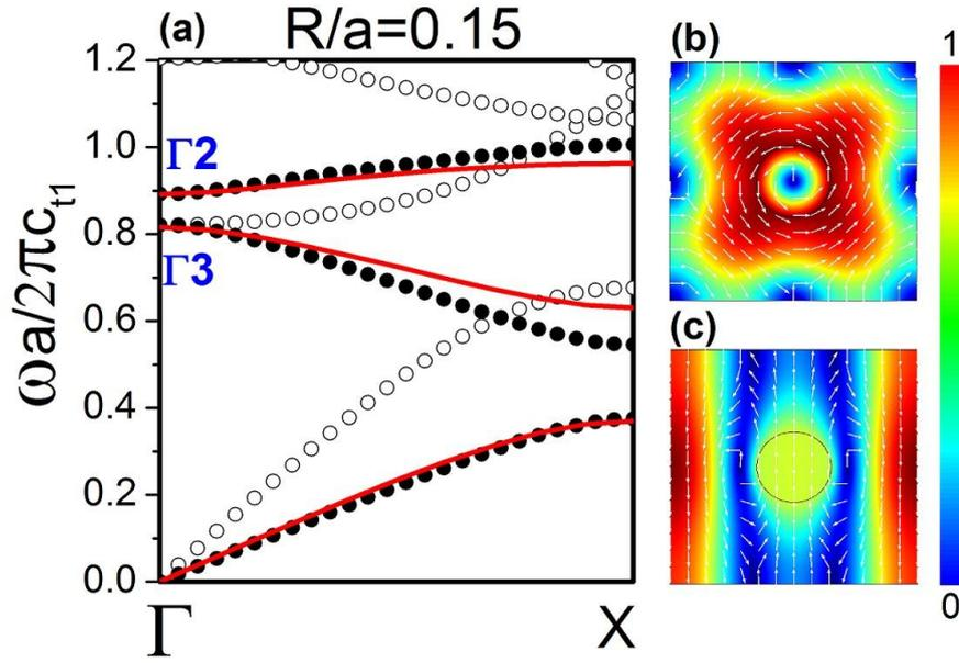
FIG. 3 (a) Band structures of the same system as shown FIG. 2, but the radius is changed to  $R/a=0.15$ . (b) and (c) are the displacement field distributions of the eigenstates marked as  $\Gamma 2$  and  $\Gamma 3$ , respectively.
