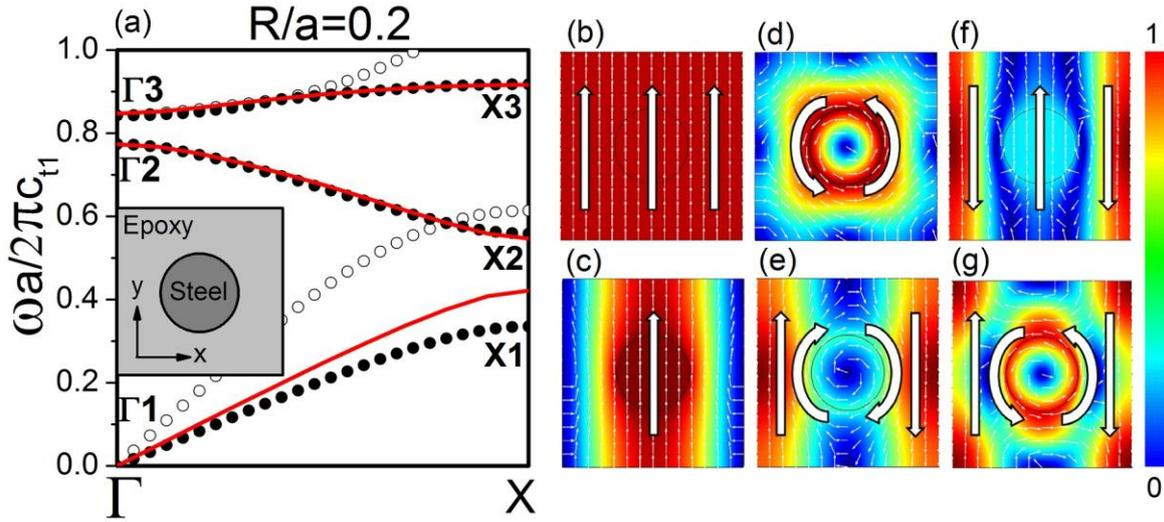
FIG. 2 (a) Band structures of a square array of steel cylinders embedded in epoxy with radius  $R/a=0.2$ . The solid dots correspond to the transverse- and rotation-related modes. The red curves indicate the dispersion curves predicted by the lumped model.
