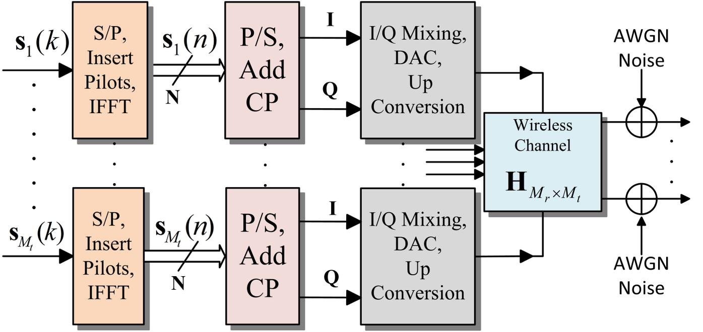
Fig. 1. MIMO-OFDM transmitter with  $M_t$  transmit branches
