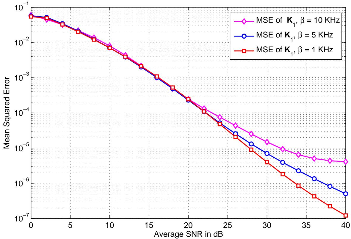
Fig. 5. MSE of IQ-imbalance matrix ( $K_1$ ) estimation for a  $2 \times 2$  MIMO system with IQ-imbalance of  $(5^\circ, 10\%)$  and different phase noise linewidths at each receiver branch
