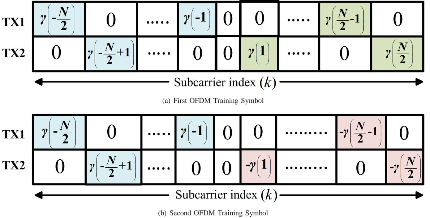
Fig. 3. OFDM preamble structure for 2 transmit antennas
