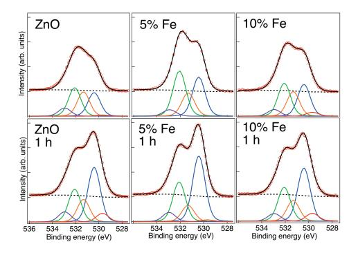
FIG. 9. XPS of O 1s before and after 1 hour of x-ray exposure. The oxygen is fitted by five peaks. Water at high BE (533 eV) is approximately the same for all samples. The hydroxide peak at 532.1 eV is higher for the 5% Fe:ZnO sample but reaches similar levels for all samples after x-ray exposure. The ZnO peak at 530.4 eV is higher for the 5% sample due to less surface adsorbed species.
