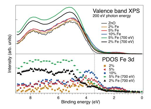
FIG. 5. Valence band photoemission with 200 eV photon energy, except when noted 700 eV. The ZnO has a VB edge at 3.4 eV BE suggesting a Fermi level close to the conduction band. Lower panel shows the partial density of states for Fe 3d. Bandgap states at 2 eV BE are not visible at high photon energies indicating their location on the surface. Fe 3d states are located deeper in the VB for more bulk sensitive measurements using 700 eV photon energy.
