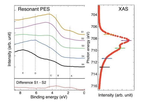
FIG. 7. (Color online) Resonant PES (left) obtained at the photon energies shown in the absorption spectra (right). Resonant features are identified for different valencies and coordinations of Fe ions. The difference between S1 and S2 is shown in the lower part to make feature B more distinct.
