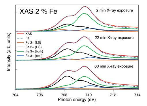
FIG. 8. Decomposition of 2% Fe:ZnO XAS for different x-ray exposure times. The Fe<sup>3+</sup> (bulk) component decreases with x-ray exposure while the  $Fe_{HS}^{2+}$  increases. The other components are relatively weak and appear unaffected by x-ray exposure.
