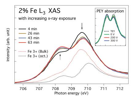
FIG. 2. XAS of 2% Fe:ZnO after different x-ray exposure times. The intensity of the main peak,  $Fe^{3+}$ , decreases as the intensity of the pre-edge peak corresponding to  $Fe^{2+}$  increases. The inset shows the partial absorption of 5 % Fe obtained after a long x-ray exposure time. The partial absorption indicates that the  $Fe^{2+}$  fraction is higher close to the surface.
