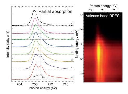
FIG. 6. Partial Fe L<sub>3</sub> absorption (left) and VB RPES (right) of 5% Fe:ZnO. The partial absorption is obtained by taking a slice from the RPES spectrum at the BE corresponding to the base line of the absorption spectra (A1 - A8). Four different components are identified as  $Fe_{LS}^{2+}$ ,  $Fe_{HS}^{2+}$ ,  $Fe_{HS}^{3+}$ tetrahedral and  $Fe^{3+}$  octahedral with peak positions at P1, P2, P3, and P4, respectively.
