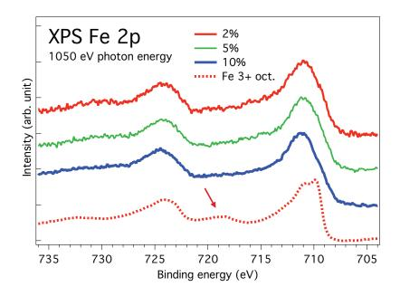
FIG. 1. Fe 2p XPS for different Fe concentrations. A reference  $Fe^{3+}$  spectra (red dashed) is also presented. The arrow indicates the location of a satellite structure which can be used for distinguishing between  $Fe^{3+}$  and  $Fe^{2+}$ . All Fe:ZnO spectra indicate a mixed  $Fe^{3+}/Fe^{2+}$  state.
