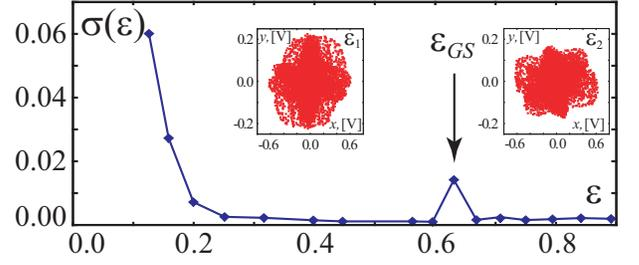
FIG. 3: (Color online) The experimental characteristic  $\sigma(\varepsilon)$  for two unidirectionally coupled klystron generators. The correlation plots  $y$  vs.  $x$  are shown in the frames for  $\varepsilon_1 = 0.10$  and  $\varepsilon_2 = 0.89$ , respectively.
