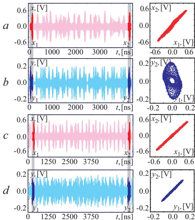
FIG. 4: (Color online) The selected fragments of time series and corresponding to them correlation plots. Figures *a* (drive) and *b* (response) correspond to the coupling strength  $\varepsilon_1 = 0.10$ , whereas *c* (drive) and *d* (response) — to the coupling strength  $\varepsilon_2 = 0.89$
