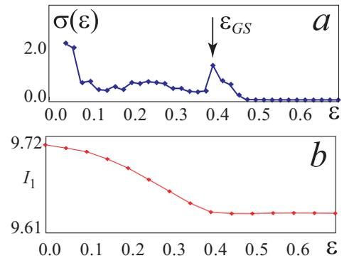
FIG. 5: (Color online) (a) The characteristic  $\sigma(\varepsilon)$  for two unidirectionally coupled klystron generators (2) and (b) the dependence of the value of the first harmonic of the bunched electron beam current  $|I_1|$  in the response klystron oscillator on the coupling strength  $\varepsilon$ . The arrows show the GS onset in coupled microwave oscillators
