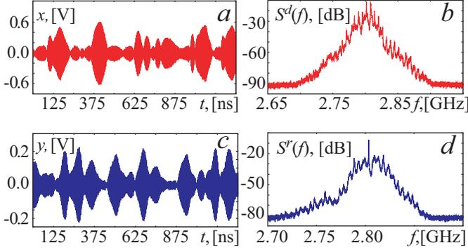
FIG. 2: (Color online) The experimentally obtained time series and power spectra. Figures *a*, *b* correspond to the drive oscillator and *c*, *d* — to the response one. Both oscillators are in the autonomous regime
