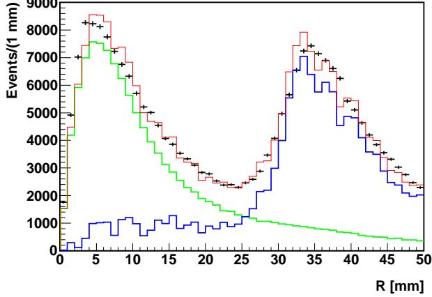
Figure 4: Distribution of the distance  $R$  between the COSY beam axis and the reconstructed point of closest approach of  $e^+$  and  $e^-$  tracks: experimental data (black crosses); simulations for  $\pi^0 \rightarrow \gamma\gamma$  (blue line), the  $\pi^0 \rightarrow e^+e^-\gamma$  decay (green line), and the sum of the two contributions (red line).
