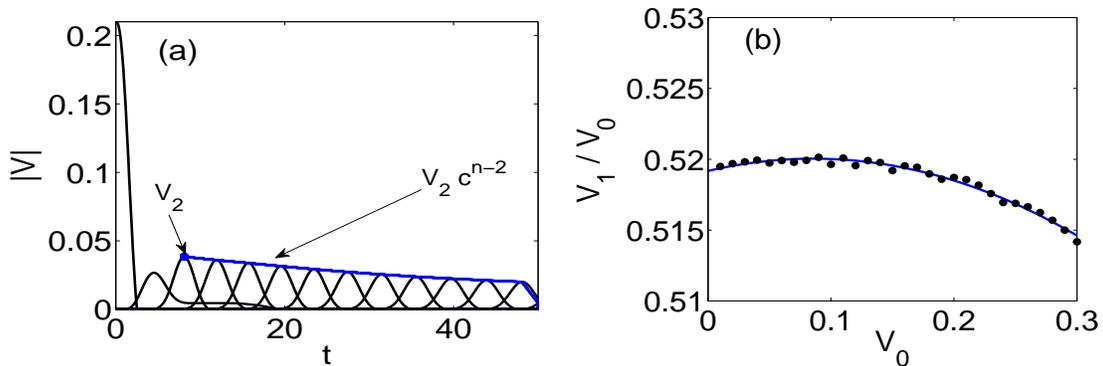
FIG. 7. (a) magnitude of the velocity of beads 0 – 12 along the  $0^\circ$  line upon being struck at a  $0^\circ$  angle. In this case, the fitting is more accurate starting at the second peak  $V_2$ . (b) The relationship between the initial striking velocity  $V_0$  and  $V_1$  for a  $0^\circ$  strike and  $30^\circ$  observation is quadratic. For this particular case, we see that  $V_1 \approx V_0/2$ .
