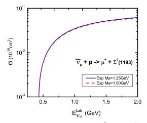
Fig. 3 (Color online) Comparison of the total cross section of  $\bar{\nu}_{\mu} + p \rightarrow \Sigma^0(1193) + \mu^+$  for different axial mass ( $M_a$ ) versus neutrino beam energy in the lab system. The *blue solid, red dashed lines* correspond to  $M_a = 1.25$  and 1.00 GeV, respectively. Other parameters are from EXP in Table 1
