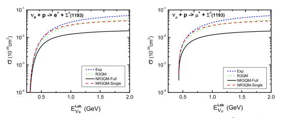
**Fig. 9** Comparison of predictions from various models for the total cross section of  $\bar{\nu}_e + p \rightarrow \Sigma^0(1193) + e^+$  (*left*) and  $\bar{\nu}_\mu + p \rightarrow \Sigma^0(1193) + \mu^+$  (*right*) versus neutrino beam energy in the lab system. The *black solid and red dashed lines* are the same as the *thin lines* in Fig. 7. The *blue short-dashed* and *green dotted lines* are from "EXP" and "R3QM" models, respectively
