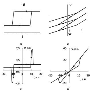
Fig. 1. Schematically view of *a* - current dependence of differential resistance R(I) for self-switching magnetic structures in <sup>7-10</sup>, *b* - corresponding this dependence divergent VAC, *c* - correct dependence R(I) for self-switched structure with parameters  $f_0=1$ ,  $\varphi=1$ ,  $\alpha=10$ ,  $\beta=10$  and *d* - corresponding Fig. 1*c* view of VAC with hysteresis.
