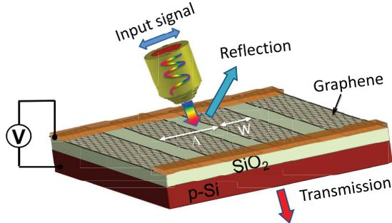
FIG. 1. Schematic illustration of the electro-optical graphene ribbon-based plasmonic switch in mid-infrared wavelengths. The graphene ribbon array has the width of  $w$  and period of  $\Lambda$  on top of the  $\text{SiO}_2/\text{p-Si}$  substrate.
