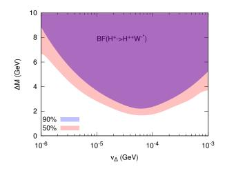
FIG. 2: Branching fraction of  $H^{\pm} \to H^{\pm\pm}W^{\mp*}$  in the  $v_{\Delta} - \Delta M$  plane for  $M_{H^{++}} = 300$  GeV. The purple and pink regions denote the parameter space where  $BF(H^{\pm} \to H^{\pm\pm}W^{\mp*})$  is greater than 90% and 50% respectively.
