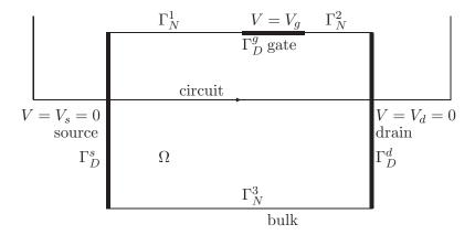
Figure 2: Representation of the transistor with partial gate
