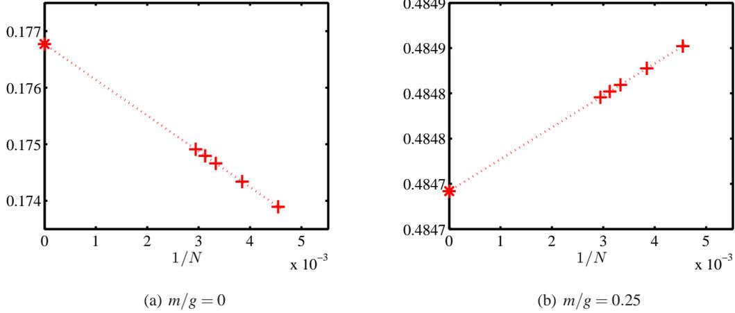
**Figure 2:** Finite volume extrapolation of the (subtracted) condensate for  $x = 100$  in the case of massless fermions (left) and  $m/g = 0.25$  (right). We fit the results to a linear function in  $1/N$ , shown by a dashed line. The extrapolated value is indicated by a star.
