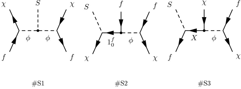
**Figure 6:** Different decompositions (Feynman diagrams) for the operator  $\chi\chi ffS$ .  $\phi$  is a scalar and  $X$  a fermion that has the quantum numbers of the external fermions  $f$ .  $\phi$  corresponds to the mediators in Fig. 3.
