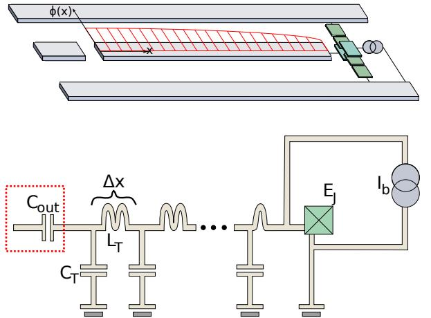
FIG. 1. (Color online) A schematic (top) and a circuit diagram (bottom) of the system. In the upper picture the fundamental normal mode of the flux is sketched. In the circuit diagram, the transmission waveguide resonator is described as a chain of capacitors and inductors. The resonator is shunted by a current biased Josephson junction. In the dashed (red) box, we couple capacitively to fields outside of the device.
