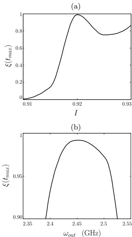
FIG. 6. (Color online) In (a) we show the detector efficiency as a function of  $I$  for fixed  $\omega_{out} = 2.45$  GHz, which is the energy-splitting between the two bound states at  $I = 0.92$ . In (b) the maximal detector efficiency is plotted as a function of  $\omega_{out}$  for fixed  $I = 0.92$ . All efficiencies are evaluated at the optimal time,  $t_{max} = 84$  ns and other parameters are once again the same as in Fig. 4.
