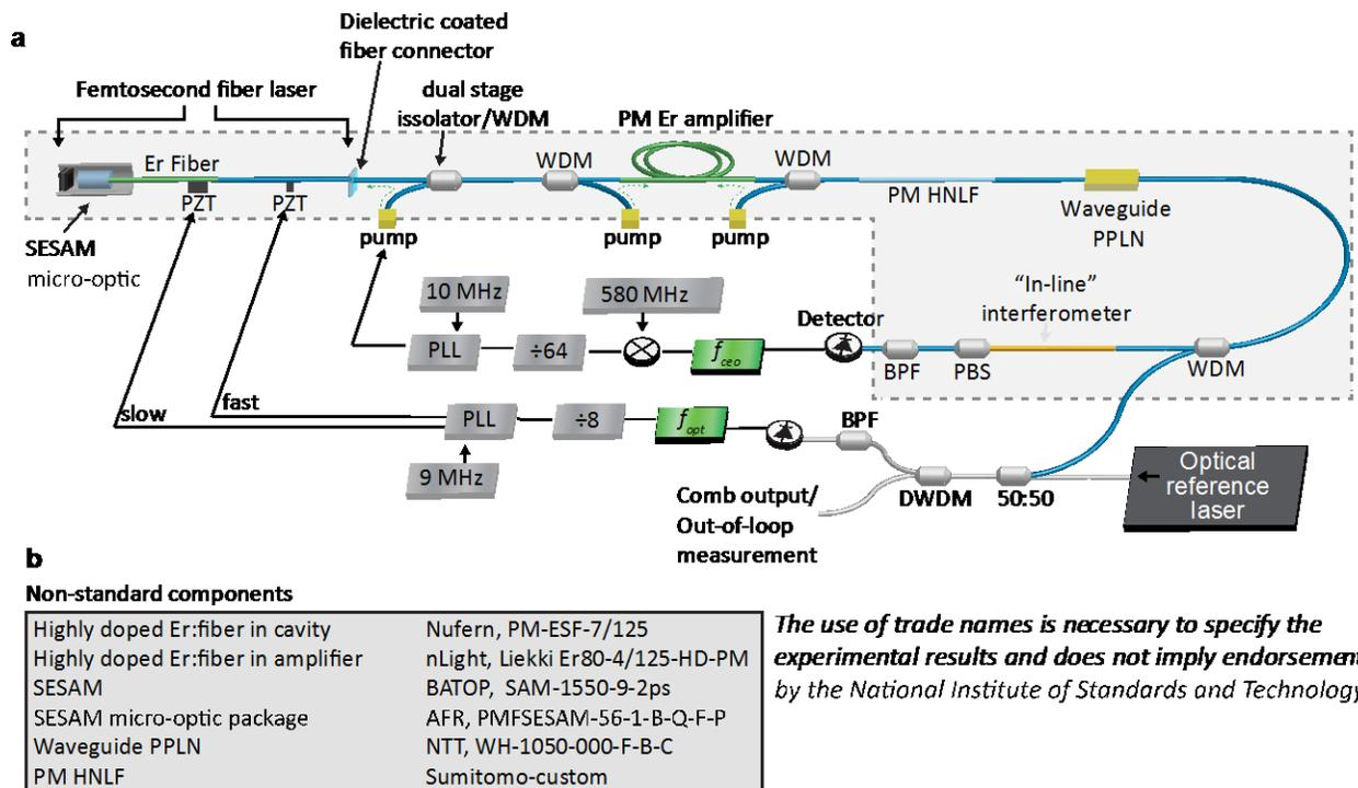
FIG. 5. (a) Fieldable coherent frequency comb design. A detailed discussion is provided in the text. The “optics package” that was shaken is shaded in light grey. PM fiber: solid blue lines, PM Er-doped fiber: solid green lines, WDM: Wavelength-Division Multiplexer, BPF: band-pass filter, PLL: phase-locked loop, PBS: polarizing beam splitter. (b) Table lists specific non-standard components used in the design.
