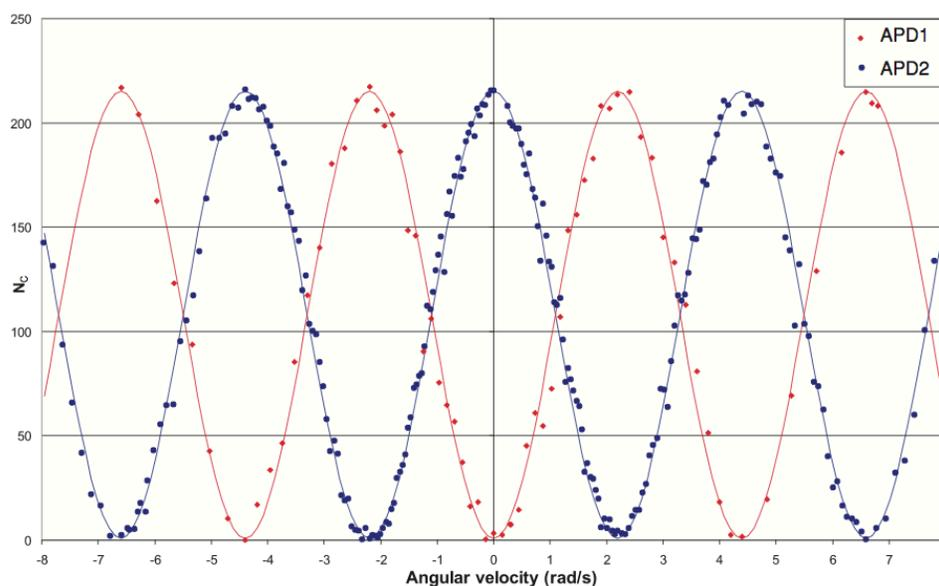
**Figure 5.** Experimental results. The interference pattern shows the Sagnac effect with visibility up to  $(99.2 \pm 0.4)\%$ . Each point corresponds to the photon number count  $N_c$  for a 300 ms integration time at a given angular velocity  $\Omega$ . We can note that  $\Omega_{n\pi} = n2.2 \text{ rad s}^{-1}$ , corresponding to formula (2).
