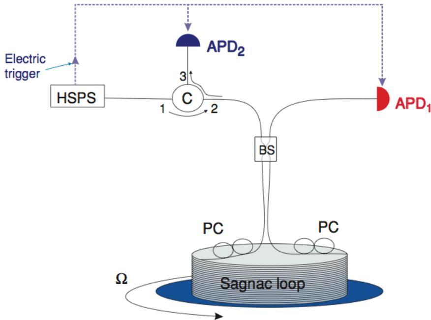
**Figure 3.** Experimental setup. Optical fibres are represented in continuous line, and electric trigger in slash-line. HSPS: heralded single-photon source. C: circulator. BS: beam splitter. APD<sub>1,2</sub>: InGaAs avalanche photodiodes. PC: polarization controllers. The 550 meters fibre optics loop is on a plane rotating at an angular velocity  $\Omega$ .
