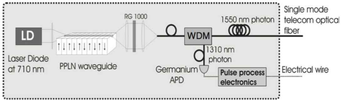
**Figure 4.** Scheme of the heralded single-photon source (HSPS). It has an electrical output which heralds the presence of a single photon in the optical fibre output. The filter (RG 1000) after the waveguide discards the remaining pump photons while the wavelength demultiplexer (WDM) separates the pairs regarding the wavelength of the photon. The 1310 nm are detected using a Ge APD in order to herald their partner photon at 1550 nm in the fibre output.
