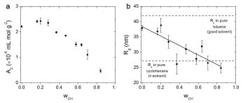
FIG. 1. Static light scattering of polystyrene in CH/CHB mixtures. (a) Changes in solvent quality, and (b)  $R_g$  of 900,000 g/mol polystyrene in the solvents used in this study. In (b), the solid line is a least-squares fit of the change in  $R_g$  as a function of  $w_{CH}$ . Literature values of  $R_g$  in a good solvent (pure toluene) and a theta-solvent (pure CH) are provided for reference [Fetters, et al. (1994)].
