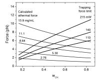
FIG. 6. Operating regime for rupture force measurements. The athermal force limit is calculated from the DLVO and Asakura-Oosawa potential. The maximum trapping force was determined from the drag calibration method for laser powers of 110, 140, and 215 mW.
