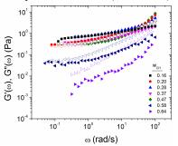
FIG. 8. Linear oscillatory frequency sweep dataset for gels with  $w_{CH} = 0.16, 0.20, 0.28, 0.37, 0.47, 0.58, and 0.64$ . Closed symbols represent G' and open symbols represent G".
