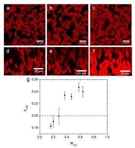
FIG. 7. Sedimentation of gels ( $\phi_{gel} = 0.20$ ) at different solvent compositions. (a-c), Representative 2D *x-y* plane CLSM images of gels with  $w_{CH} = 0.16$ , 0.37, and 0.64; images are taken at z = 10 µm; (d-f), representative 2D *x-z* plane (z = 0.30 µm) CLSM images of gels at the same solvent compositions; (g),  $\phi_{wall}$  as a function of  $w_{CH}$  estimated from the number of particles in the *x-y* plane at z = 10 µm. Error bars shown are standard deviations of the mean.
