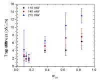
FIG. 5. Trap stiffness of PMMA particles ( $2a = 2.7 \mu m$ ) in mixtures of CH and CHB as a function of  $w_{CH}$  measured using the drag calibration method at 110, 140, and 215 mW. Error bars are 95% confidence intervals.
