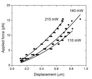
FIG. 4. Applied force as a function of displacement from drag calibrations at  $w_{CH} = 0.84$  as a function of laser power. There are three replicates at each laser power. Lines are quadratic fits to the data.
