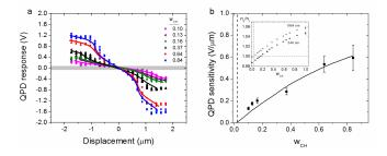
Figure 3. (a) QPD response to the displacement of PMMA particles ( $2a = 2.7 \mu m$ ) from an optical trap in mixtures of CH and CHB. The QPD response must be outside the gray box to be detectable. (b) QPD sensitivity as a function of  $w_{CH}$ . Inset is refractive index contrast as a function of  $w_{CH}$  measured at 546 nm and shifted to represent contrast at trapping wavelength (1064)
